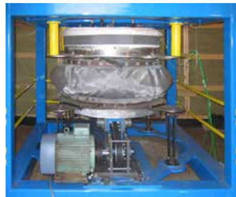
High cycle fatigue test rig.
