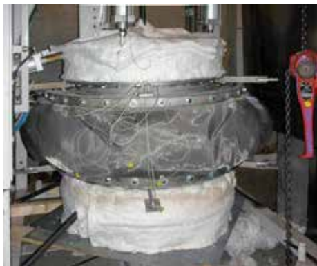
Low cycle fatigue test rig.
