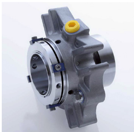
Cartex-DN double mechanical seal with connections and integrated pumping device. The viscosity of the barrier/buffer medium is recommended to be max. ISO VG 5.
